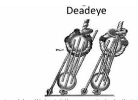
A rounded wood block encircled by a rope or an iron band and having holes to receive the lanyard that is used especially to set up shrouds and stays. The Rydal Hall deadeye is believed to have been made of lignum vitae, an extremely hard tropical wood that is 1.23 times heavier than water. It's hardness and weight contributed to its longevity at the shipwreck site.
